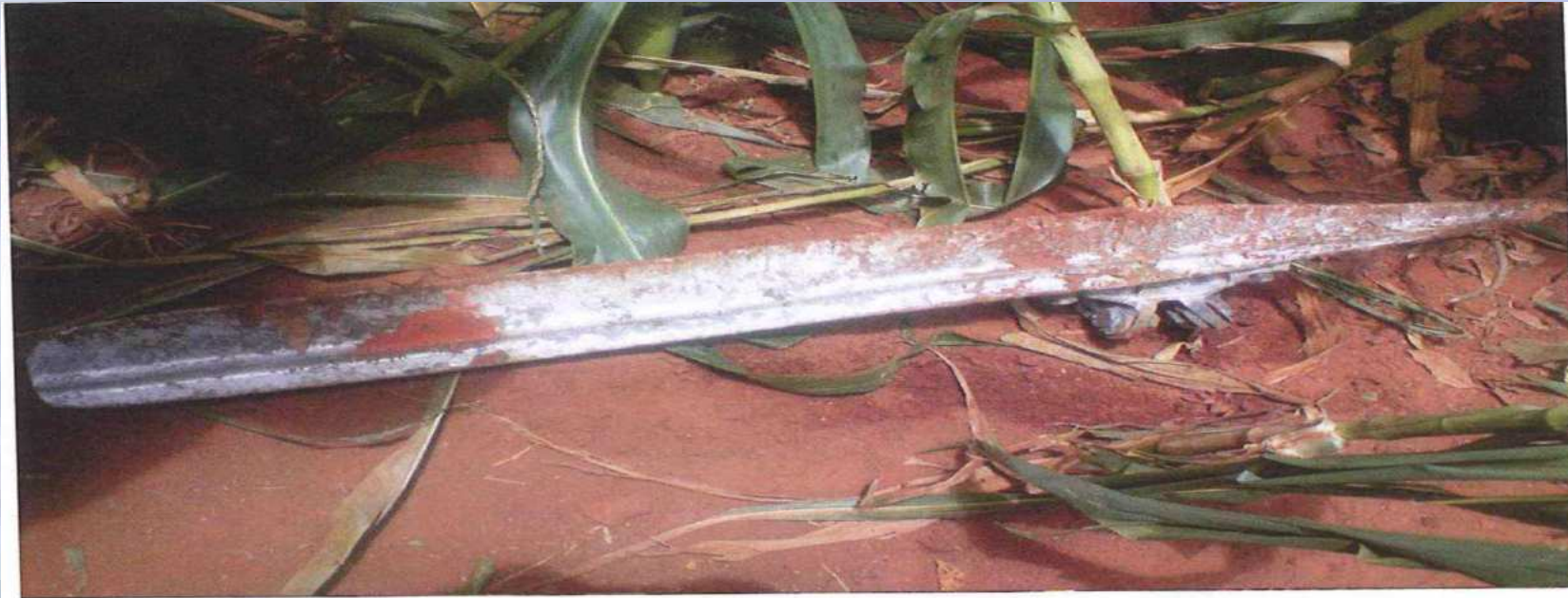
Figure- 1: LH2 Tank Fore-end Ring with lower stub adapter bracket
